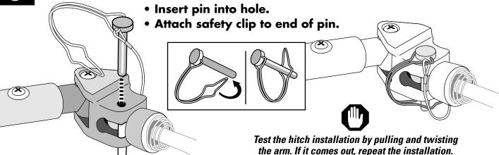
If the lanyard interferes with any moving parts, it can be cut and removed from the hitch.
