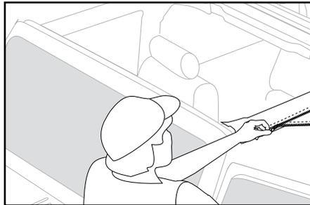
Carefully remove foam by popping out plastic fasteners.
