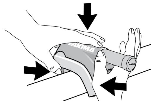
*(If the pads are not seated on the tower, the claw may not seat to the roll bar)*
