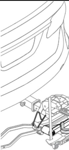
Periodically it may be necessary to adjust the tension of the swing arms. Use a 5 mm hex wrench to make the adjustment.
