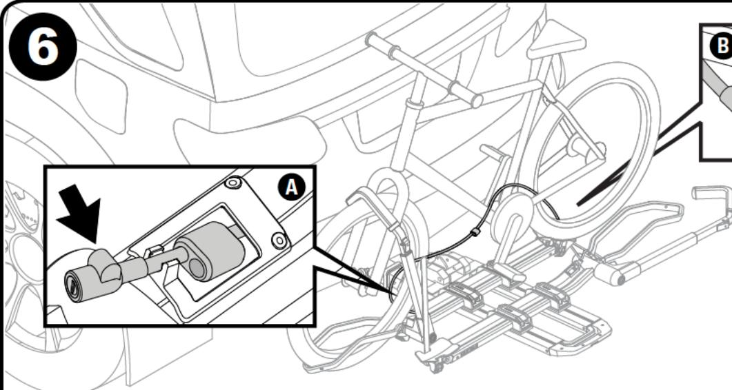
Access locking cables near the pivot arms. Pull the cable out, and pass it through one wheel, around the frame, through the other wheel, and to the lock post. Then lock it. Repeat for your other bike if applicable.
