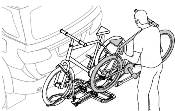
If you have bike-to-bike interference when loading two bikes, adjust trays as necessary to eliminate interference between bikes.
