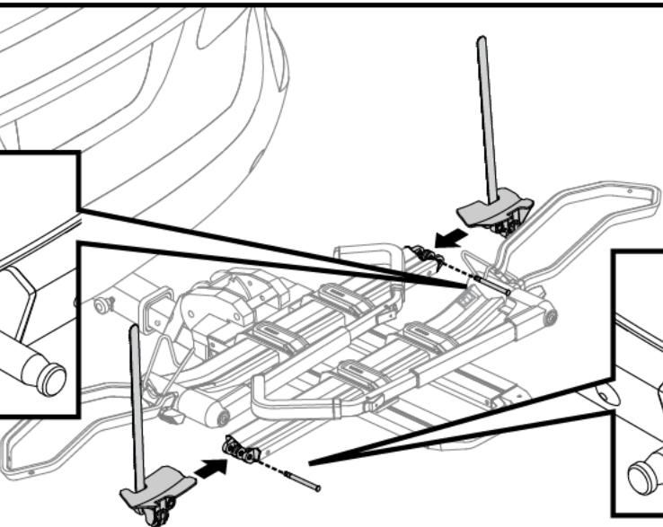
Attach the wheel cups by inserting the lock posts through the hole, front to back. Secure with e-clips.
