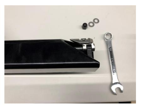
4. Re-attach acorn nut and tighten fully, do not need to re-install the washers.
