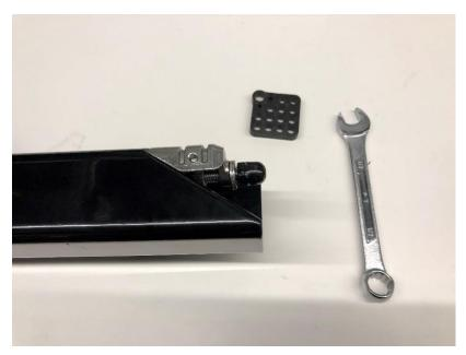
2. Remove acorn nut, washers, and wedge from long bolt.
