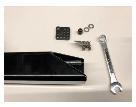
3. Insert wedge alignment insert in the gap in the wedge and re-thread onto the bolt.
